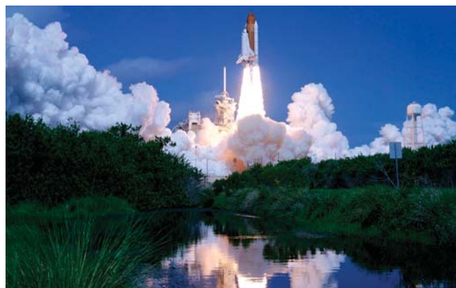
The NASA space shuttle launched on July 8, 2011, used more than 28,000 L of liquid helium. The transition from liquid to gaseous helium provided necessary pressure to the system, and the helium helped push out the combustion products formed during the liftoff.
